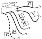
STEP 1 - Connect the **G** wire to the **G** terminal on the thermostat.
