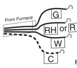
STEP 1 - Connect the R (or RH) wire to the RH terminal on the thermostat. This connects to the Heater Power.
