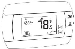
When using a heat pump with Auxiliary heat, if the heat pump cannot keep up and/or is defective, touch the MENU button, then touch PUMP; the PUMP OFF icon will come on.. The aux heat will then be your only source of heat. When the heat pump is again operational, be sure to turn the heat pump back on by touching MENU and then PUMP (off icon goes out) as the aux heat is more expensive than pump heat.
