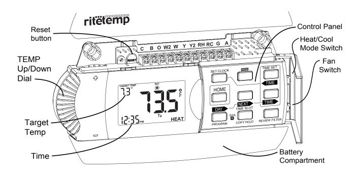
Statement of use: The 6025 can be used with - millivolt, 24V single and 2-stage conventional systems, gas/oil/electric heat, 1-stage heat pumps, 2 -stage heat pumps, zoned hot water (2 or 3 wire), zoned forced air, single and 2-stage cooling, and hybrid systems.
