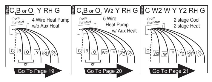
• If you combination of wires is not above you can use the wiring table on pages 24-25 to determine your connections, or call our USA support line at 1-877-505-2353 for help.
