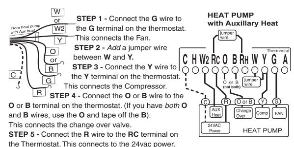
STEP 6 - Connect W or W2 to W2 on the thermostat. This connects the AUX heat.
