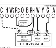
NOTE: Wires marked with the dotted line are optional.
