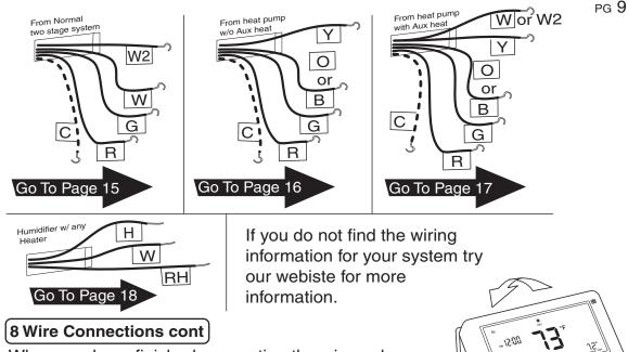
When you have finished connecting the wires, close cover and attach control unit to wall unit. Hook the top of the body onto the base, swing the body down, and snap the body onto the base.
