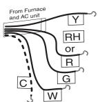
STEP 1 - Connect the Y wire to the Y terminal on the thermostat.
