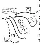
STEP 1 - Connect the G wire to the G terminal on the thermostat. This connects the Fan.
