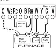
STEP 3 - Connect the G wire to the G terminal on
