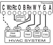
STEP 3 - Connect the W wire to the W
