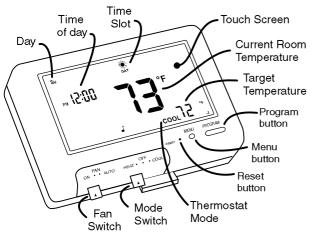
Statement of use: The GPMG8030 can be used with most 24 volt gas, oil or electric heating and air conditioning systems, single-stage heat pumps or gas millivolt heating systems. It cannot be used with 120 volt heating systems or multistage heat pumps.
