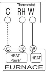
NOTE: Wires marked with the dotted line are optional.
