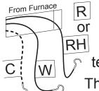
STEP 1 - Connect the R (or RH) wire to the RH terminal.
